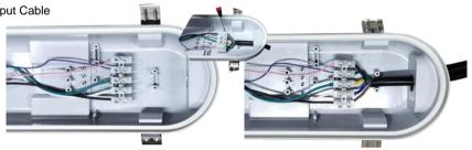
Place 5 wires Dim (-), Dim (+), Ground (PE), Neutral (N) & Line (L) in right order. Dim (-) and Dim (+) must be installed last.
